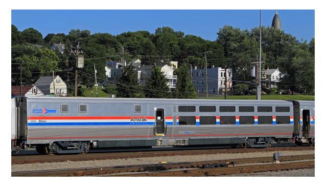
Four types of Viewliners are currently being delivered to Amtrak by CAF in Elmira, NY. These include dining cars (above), sleeping cars (below), baggage-dormitory cars with space for onboard employees and full baggage cars, which have provisions for safely handling bicycles and other awkwardly-shaped passenger belongings. The basic design is adaptable for the creation of coaches, coach-cafés and other car types. Photos by John Sesonske
