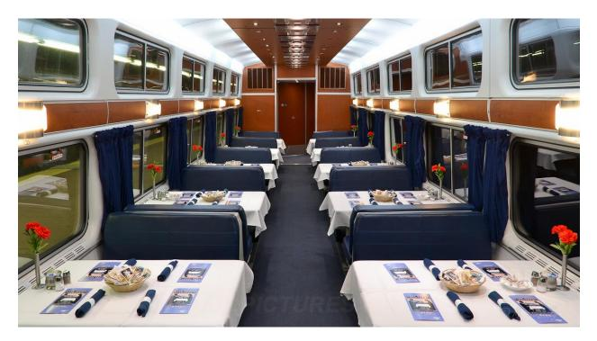
The Viewliners include a row of upper windows to create a more spacious, airy ambience than is provided by VIA's Renaissance cars, which are used on the *Ocean*. Many travellers find the Renaissance cars to be cramped, which is a result of their construction to the more restrictive clearances of the British railway system.
